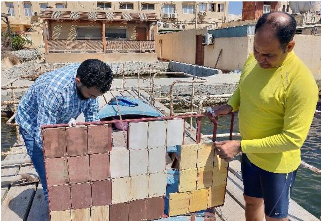
**Fig. 3 :** Steel frame with different plates.
