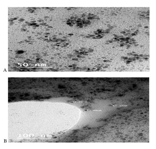
**Fig. 2.** Scanning electron microscopy of nano copper particles (A: the nano copper at 50 nanometer, B: at 100 nanometer).
