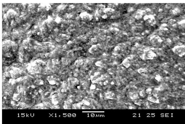
Fig. 4: SEM micrograph of silver nanoparticles
